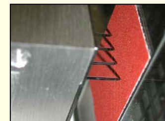
The tip shows no visible wear after 50,000 print cycles on aluminum oxide sandpaper.
