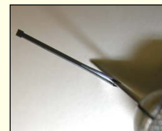
Reversibly stretching the prongs of the pin from 25µm to 200µm with a razor blade.
