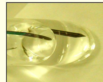
Reversibly stretching the prongs of the pin from 25µm to 200µm with a razor blade.
